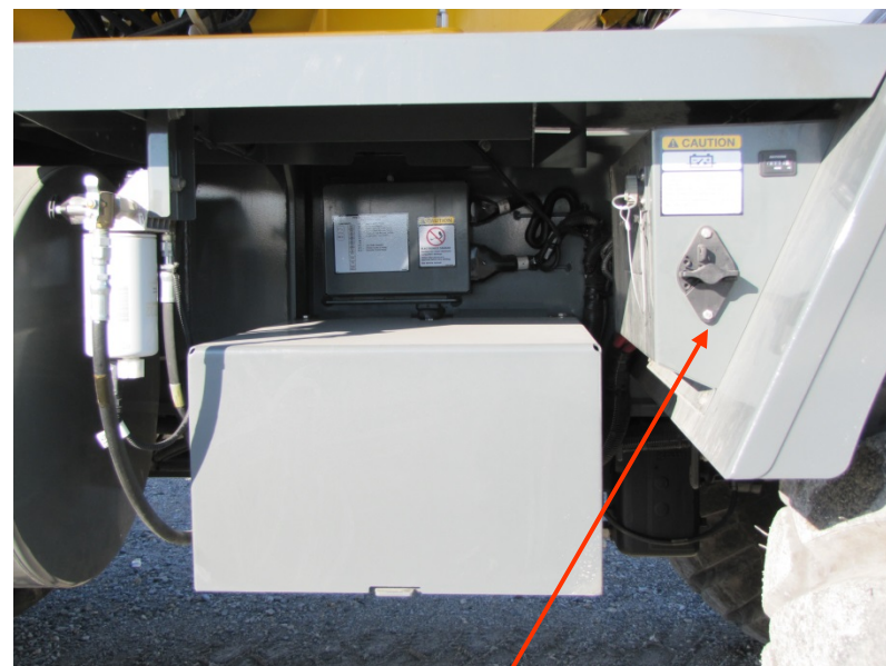
Battery disconnect switch
