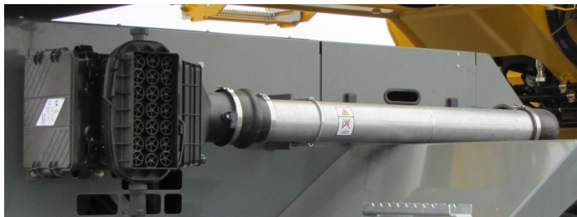
Cummins Air intake system to match E.P.A. requirements related to serialization Of engine / exhaust / air intake.
