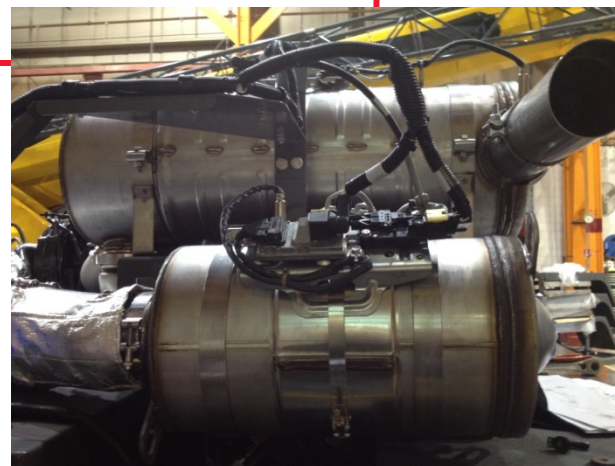
•Cummins Compact Catalyst (CCC) & Selective Catalytic Reduction (SCR) combo muffler, using Diesel Exhaust Fluid (DEF) injection to meet Tier IV FINAL emissions.
